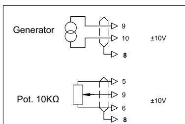
NOTE: with the potentiometer as reference signal it is necessary to connect PIN 10 with PIN 11.
