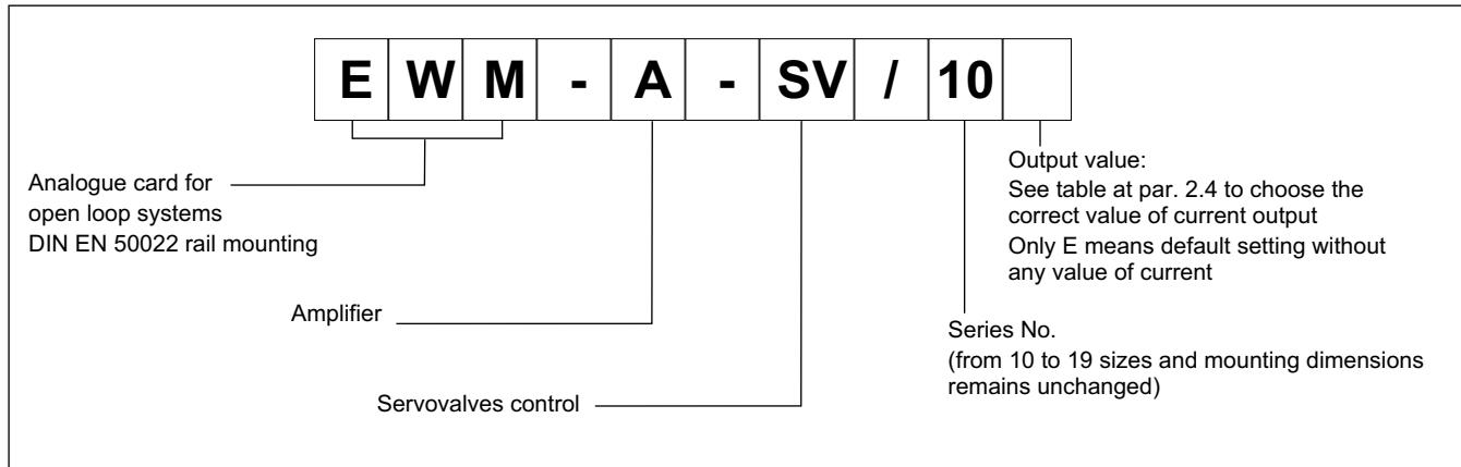
The power amplifier is controlled by an analogue input  $\pm 10$  Volt.
