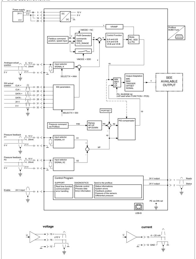
**NOTE**: If the card is configured as simple positioning control without pressure limitation then the output value is calculated just from the output of the position controller (CS) instead of apply MIN and MAX parameters. MIN/MAX are selected by the PQ\_INVERSE bit (Profibus).
